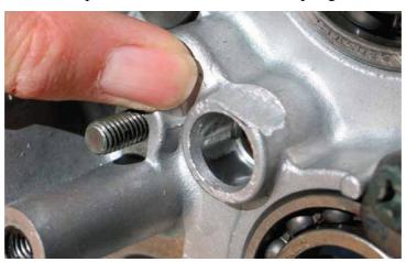
2. A small radius of material will need to be removed from the 2 output shaft selector forks to give suitable clearance to the large diameter input gears.
